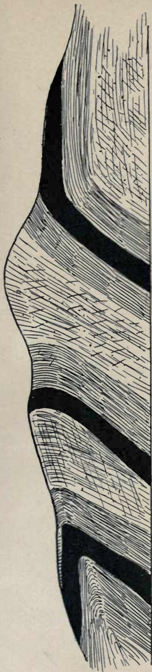
SECTION SHOWING OVERTURNED OUTCROPS.
