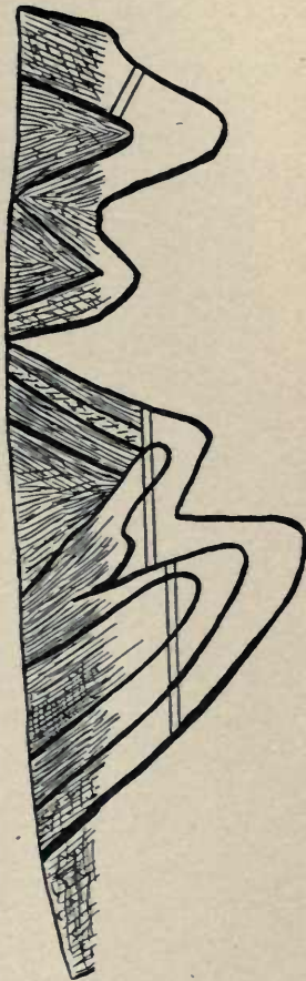
SECTION SHOWING UNDERGROUND TUNNELS CONNECTING VEINS.
